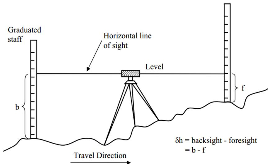
Figure 2. Spirit levelling procedure (Kemboi & Odera, 2016)
