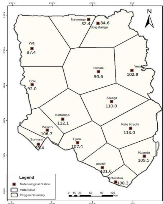
Figure 5: Thiessen polygon map showing mean annual rainfall depths in the River Volta catchment
