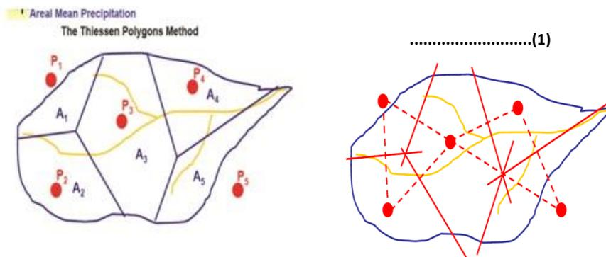
Figure 1: Steps for the determination of the Thiessen polygon method
