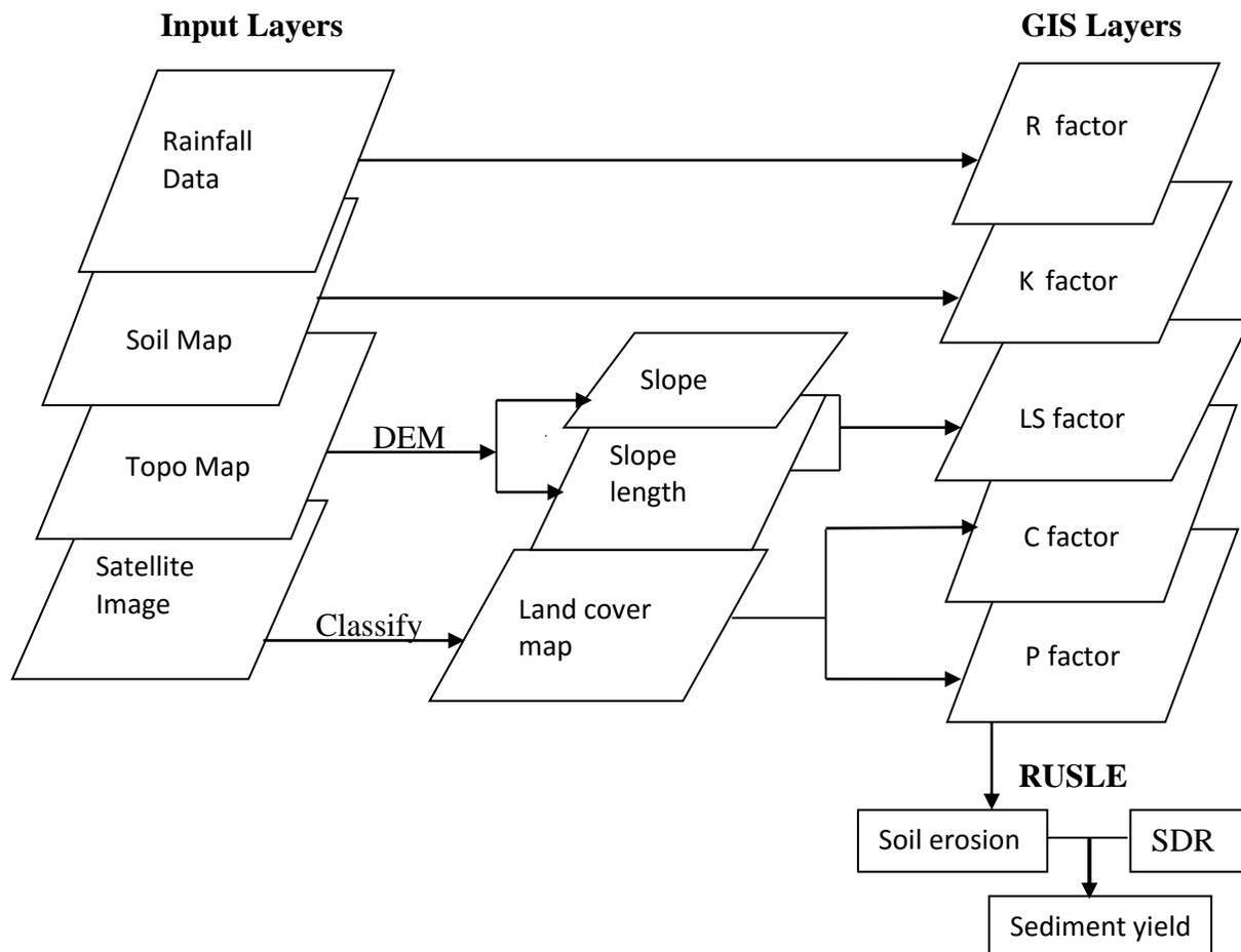
**Fig.2: Schematic chart of GIS applications to soil erosion mapping and the derivation of Sediment Delivery Ratio - SDR (Modified from Mongkolsawat et al. 1994).**
